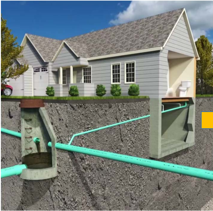
Lateral Sewers of residences and businesses
