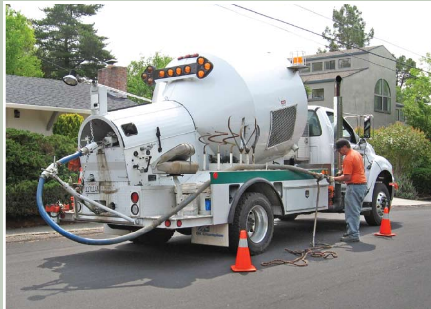
This is a power-rodding truck. It can push a flexible steel cable into pipes, with different cleaning attachments (auger, cutter blades, scrapers) on the end to cut through roots and other blockages. The majority of plugged sewers in our area are caused by roots getting into the pipes.
