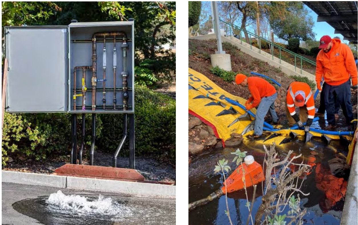
Figure 4.16: Spill Estimation Simulator and Containment Dam Deployment at CSO Facility
