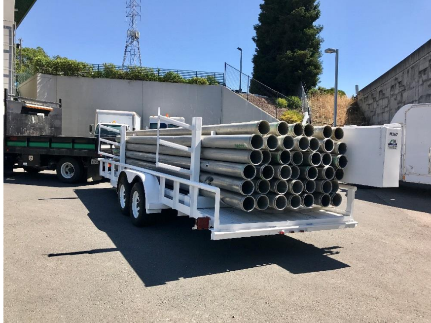
Figure 4.23: Emergency Response Pipe Trailer
