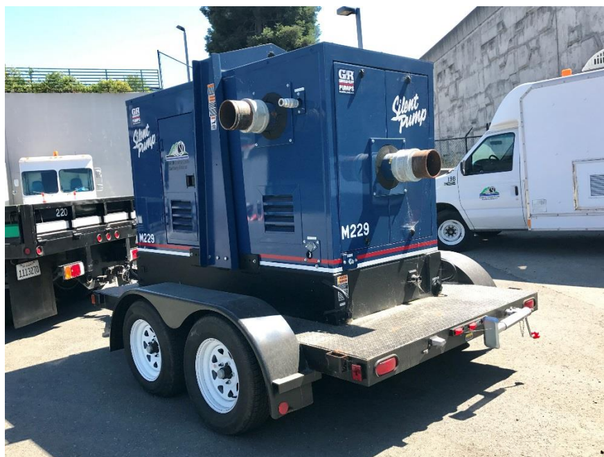
Figure 4.26: Gorman-Rupp Bypass Pump at CSO
