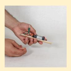
Insert the paperclips into the remaining lever nut openings, on either side of the battery.
