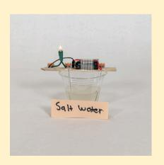
Place your conductivity meter onto the cup's rim to submerge the paper clips in solution. Make sure that the paper clips do not touch underwater.
