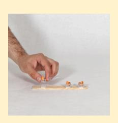
Remove the other adhesive covers on your mounting tabs. Take 3 lever nuts and secure them to each mounting tab.
