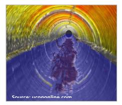
profiling, sonar, hydrogen sulfide monitoring, and visual walk-over surveys are recommended to assess the condition of large diameter sewers. Inspection information can be used to ensure replacement of pipelines prior to failure and appropriate timing of replacement.
