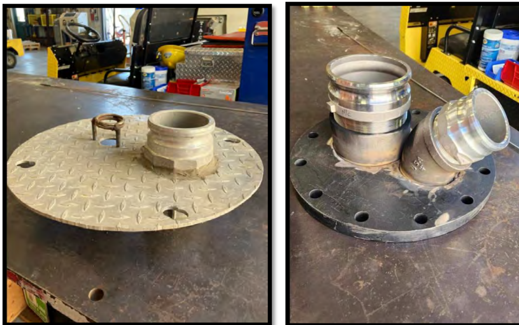
(Left – old adaptor plate, Right – New permanent flange)
