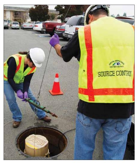
Wastewater from the collection system is sampled before it reaches the treatment plant. CCCSD employees place a device that automatically collects water samples from the sewer every 15 minutes over a 24-hour period. The samples are tested at the laboratory for metals (such as mercury, copper, and lead), oil and grease.
